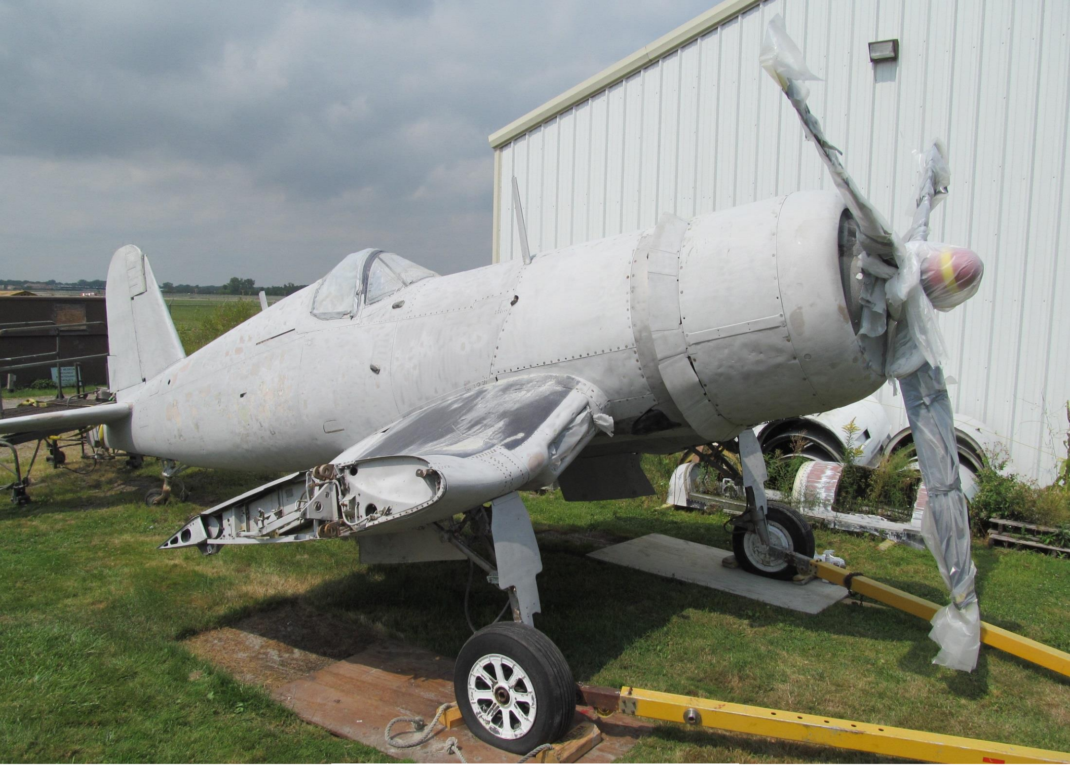
After Paint Stripping
