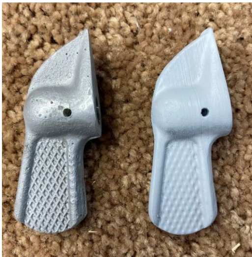
Centerline Fuel Tank Control Lever
