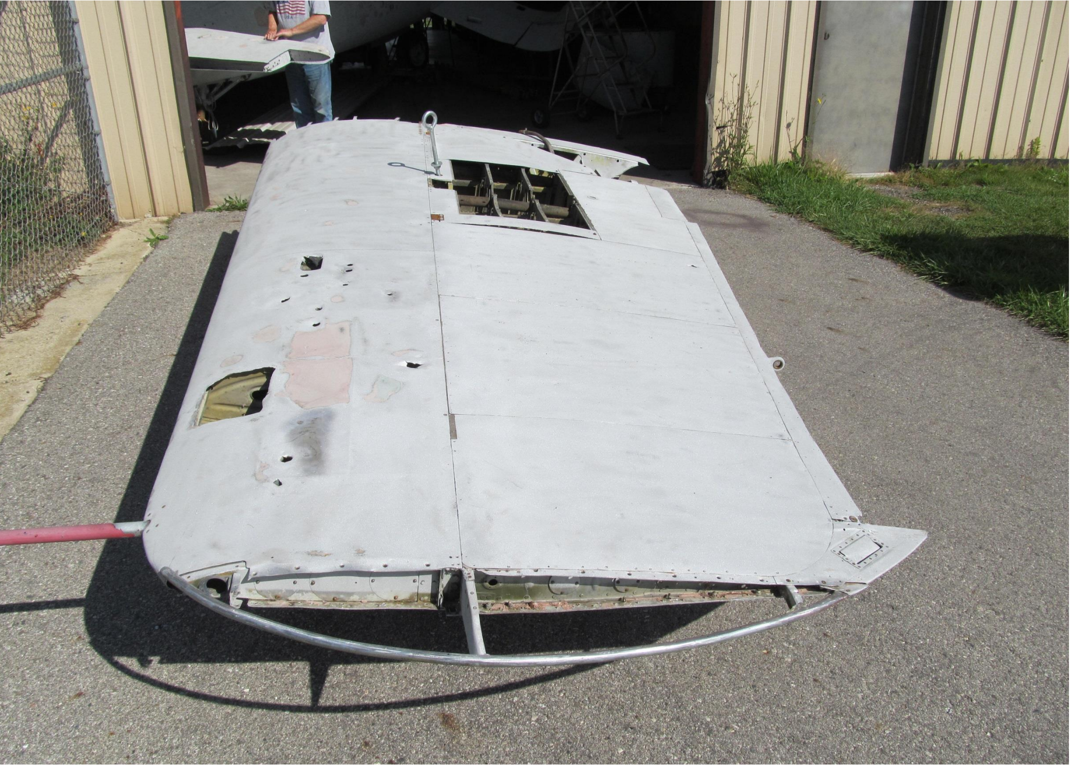
OB Wing Damage and Missing Tip After Paint Stripping 36
