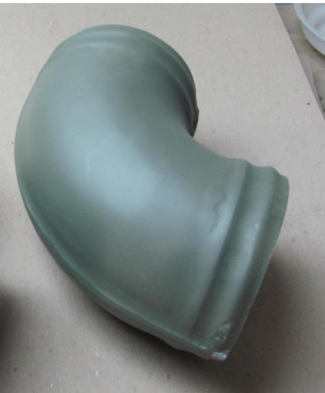
New Engine Air Induction Ducts Fabricated
