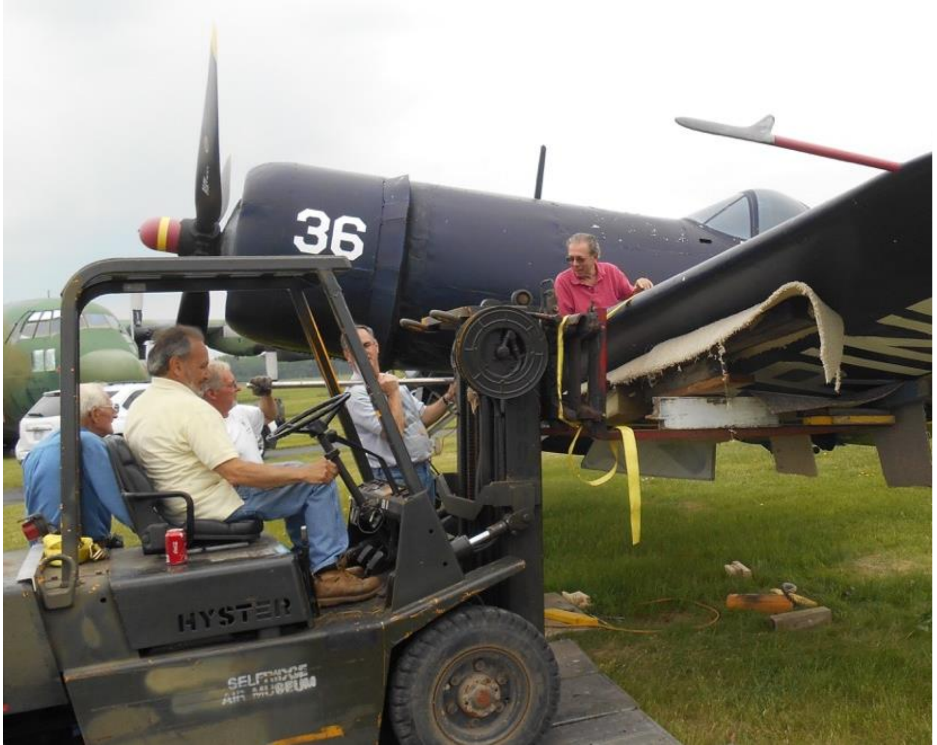
Wing Pin Removal w/ Rod & Sledge Hammer 2015
