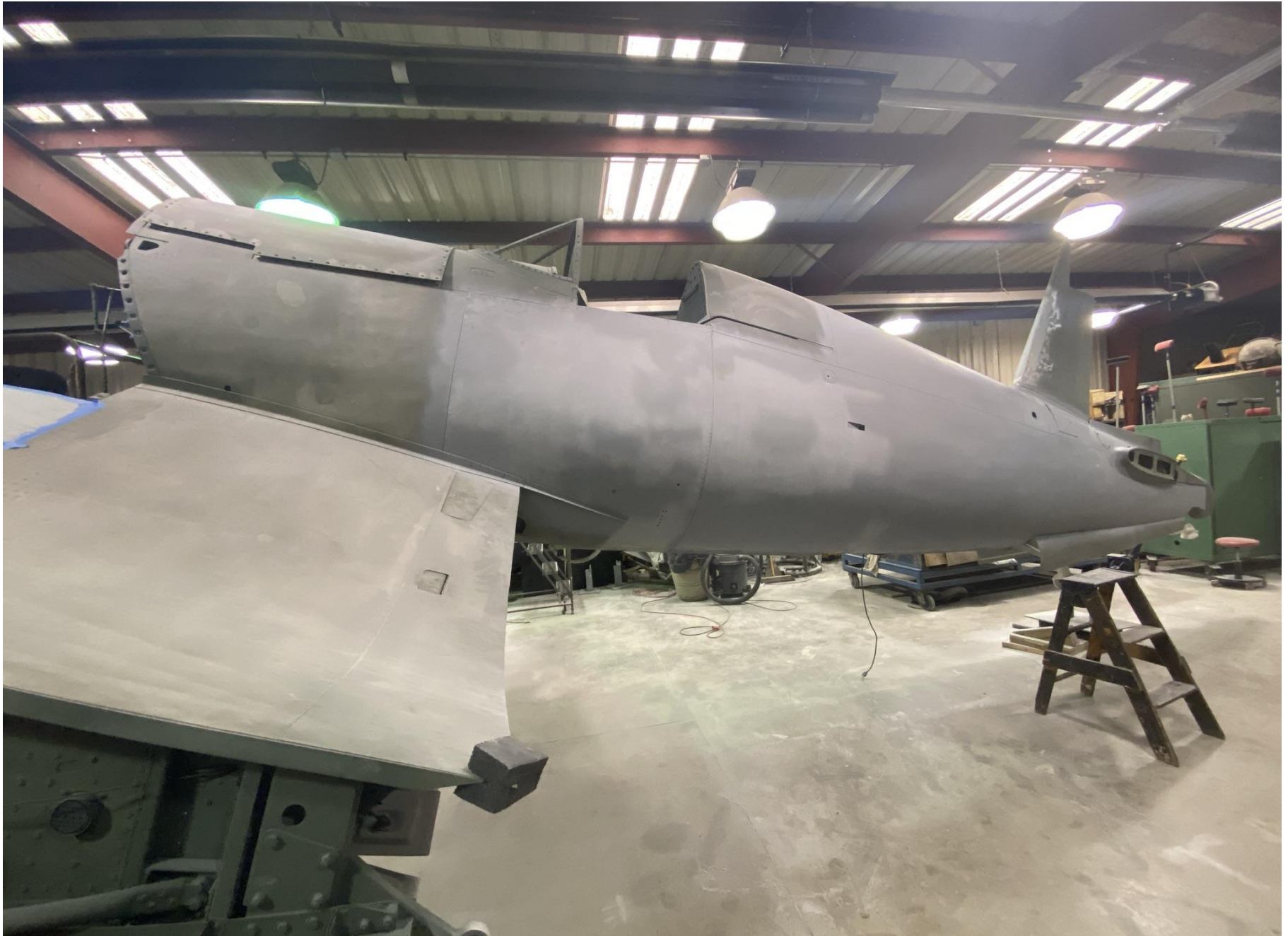
Bullet Holes and Damage Repaired, Fuselage Smoothed & Primed Prior to Painting
