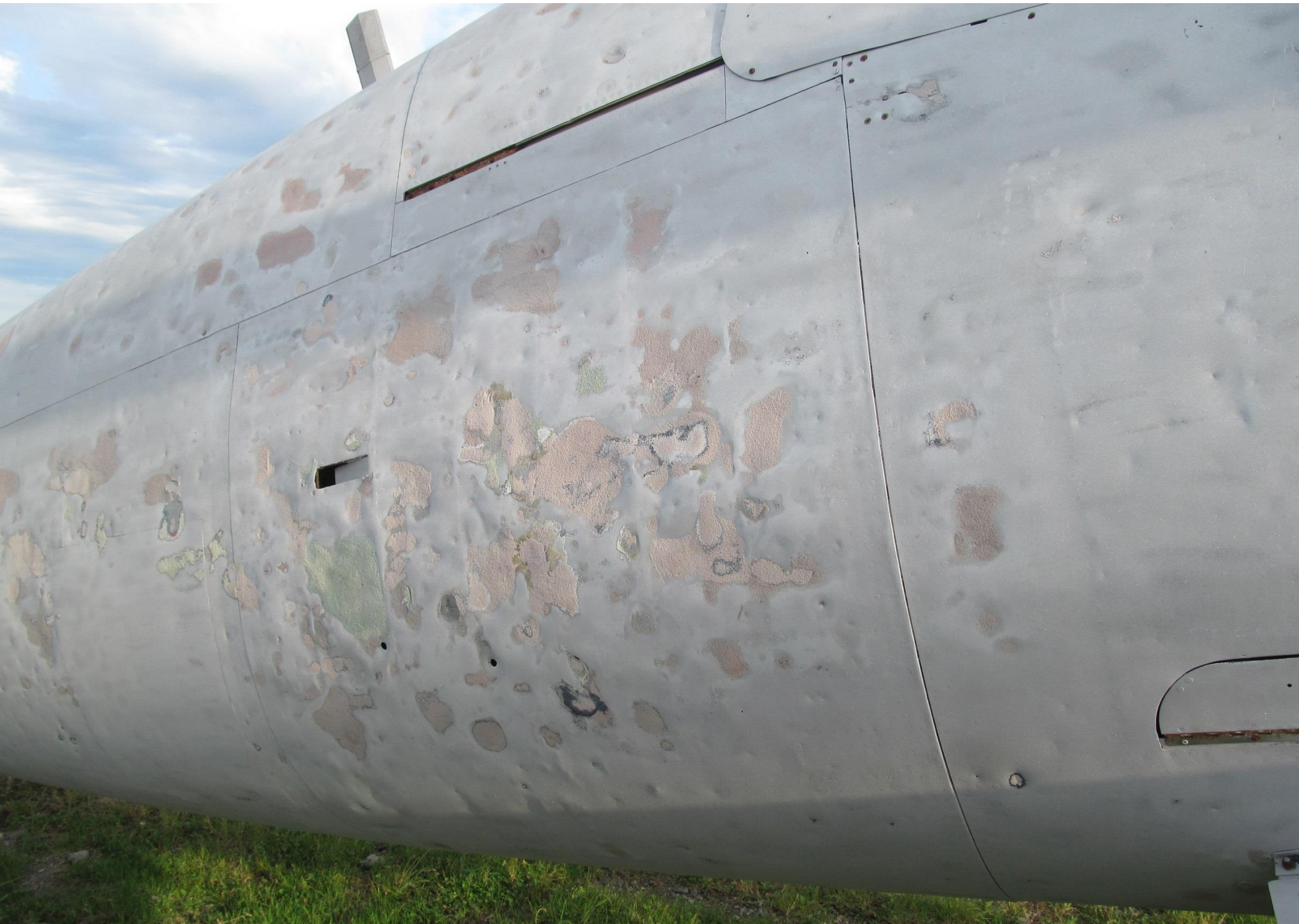
Right Fuselage Side “Bondo” Hole Patches
