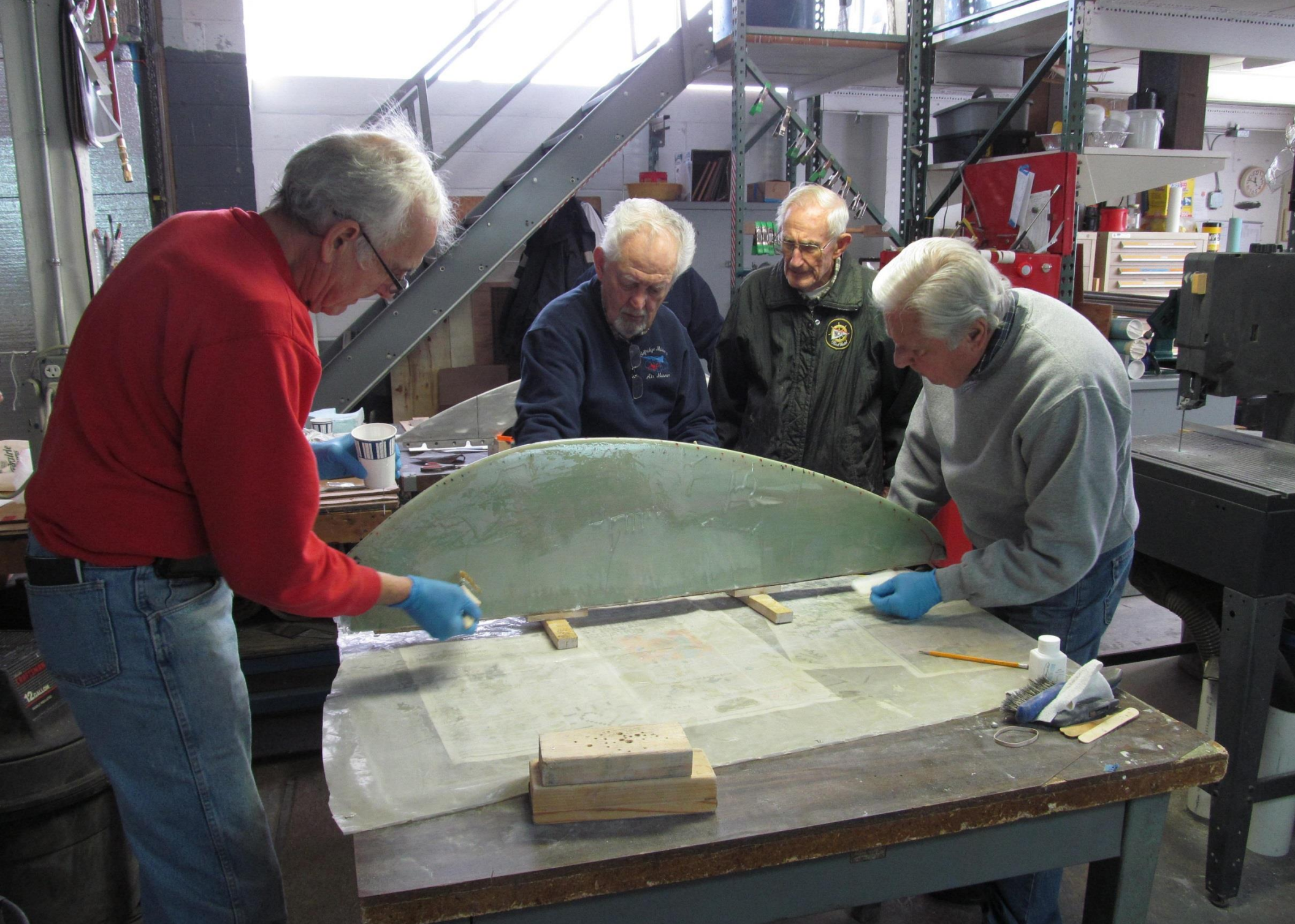
Building New Left Wing Tip From Fiberglass & Epoxy 27
