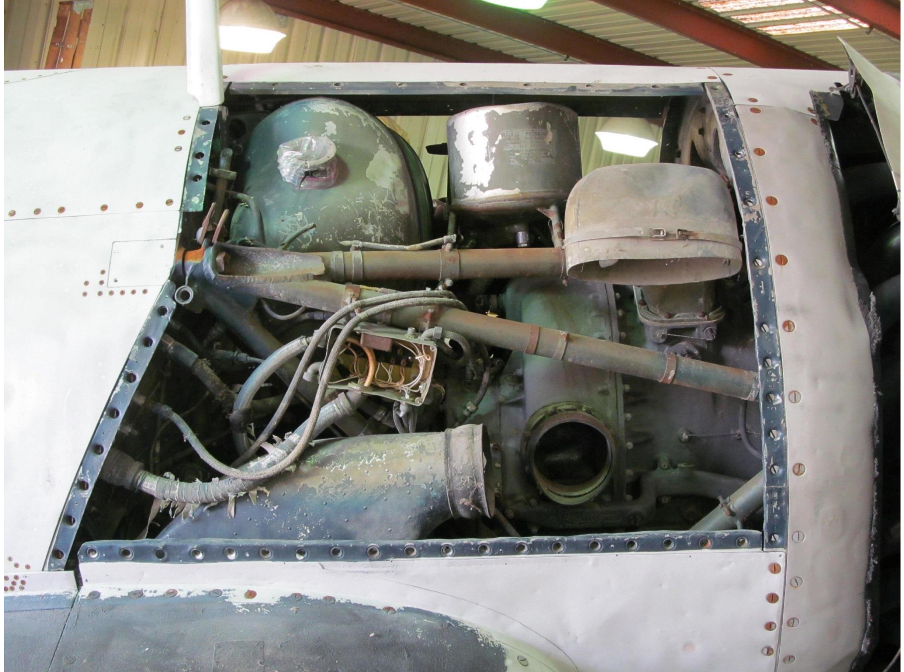
Engine Accessory Section: Four of Eight Air Induction Ducts Missing
