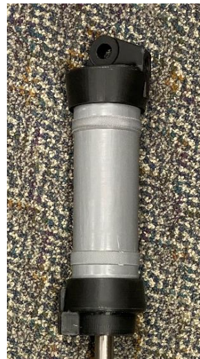
Landing Gear Door Hydraulic Cylinders
